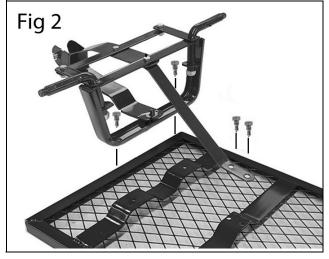
3. Slide the axle braces, over the ends of the rear axle and attach the assembly to the trolley bed using the bolts, flat washers and lock-nuts supplied as shown in Fig.3.
